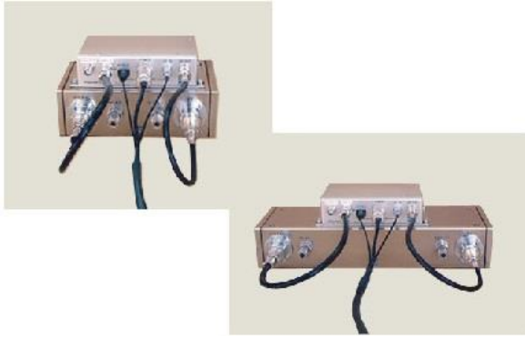
Digital ion chambers (Designed specific to SPring-8) for incident beam and IO (left) and for transmission beam and I (right).
